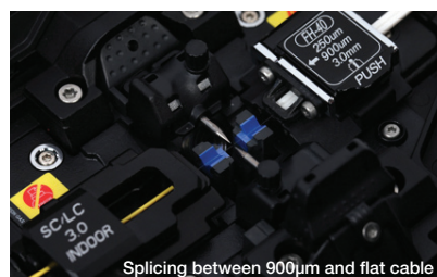
Splicing between 900µm and flat cable
