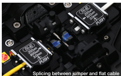
Splicing between jumper and flat cable
