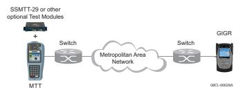
Loopback mode allows the specified Ethernet port to send incoming Ethernet frames back to the sender for end-to-end testing. Performing loopback tests is a common means of verifying the roundtrip delay of the network. The Ethernet loopback functions have been designed to emulate those used in traditional T-carrier networks. Manual mode immediately sets the port into loopback, whereas Responder mode allows the far end unit to send loop up and loop down commands.
